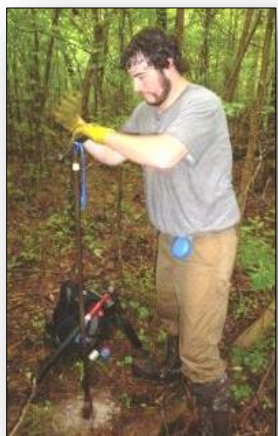
Josh Chandler uses a soil auger to assess below-ground soil conditions at different depths before harvesting.
