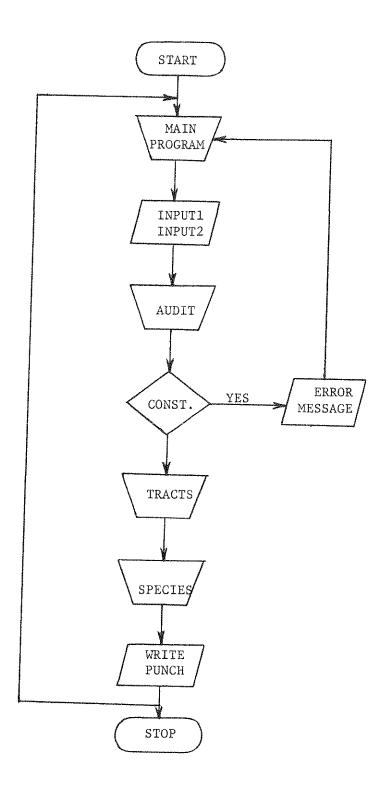
Figure 1. Flow chart showing linkage between main program and subroutines.
